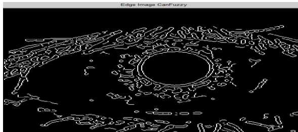
Fig.5.7 Detection of edges using Fuzzy-Canny logic.
