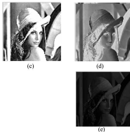
Fig. 7. (a) A low contrast Image. (b) Image after contrast stretching (c) image after histogram equalization. (d) image after negative image transformation. (e) image after power law transformation.
